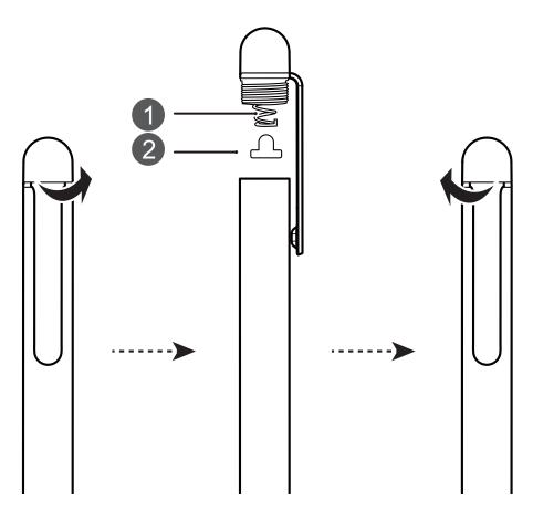
Before using your M-Pen lite for the first time, unscrew the pen cap, take out the red insulation pad beneath the pen cap, and then screw in the pen cap, as shown in the preceding illustration. You are now ready to use your M-Pen lite.
